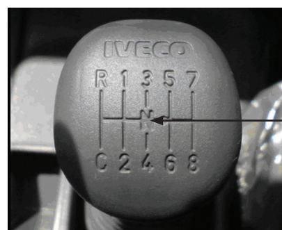
Range Change Control located in Neutral Position
