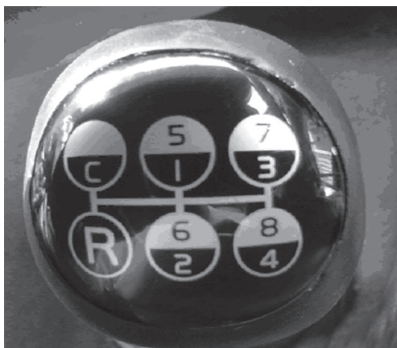
8 Speed Range Change Transmission Shift Pattern Arranged 'Four-over-Four'
