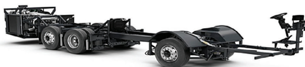
Example of a bus chassis and a rear mounted engine
