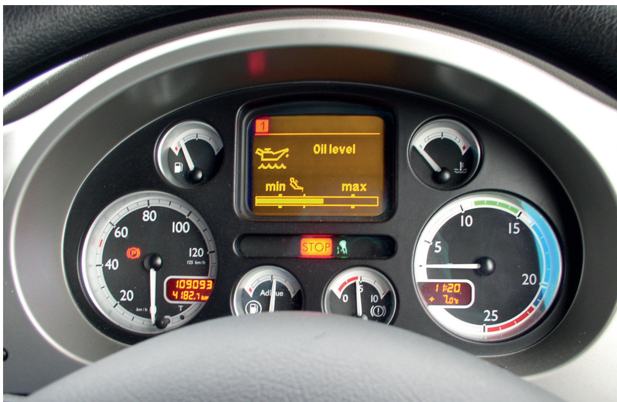
Example of Tachometer blue zone where the exhaust brake effect is maximized.
