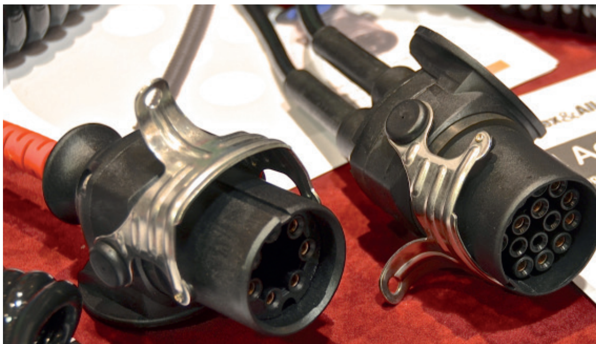
Example of EBS cable (ISO7638) with locking rings.
