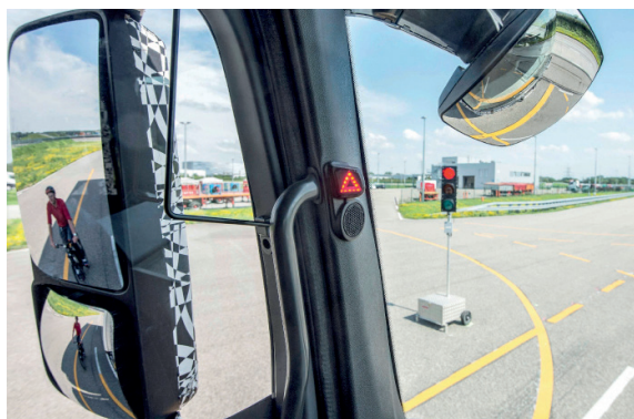
Example of visual and acoustic warning of 'blind-spot' obstruction
