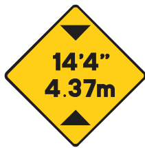
Low bridge ahead
