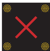
Tunnel Lane Closed
